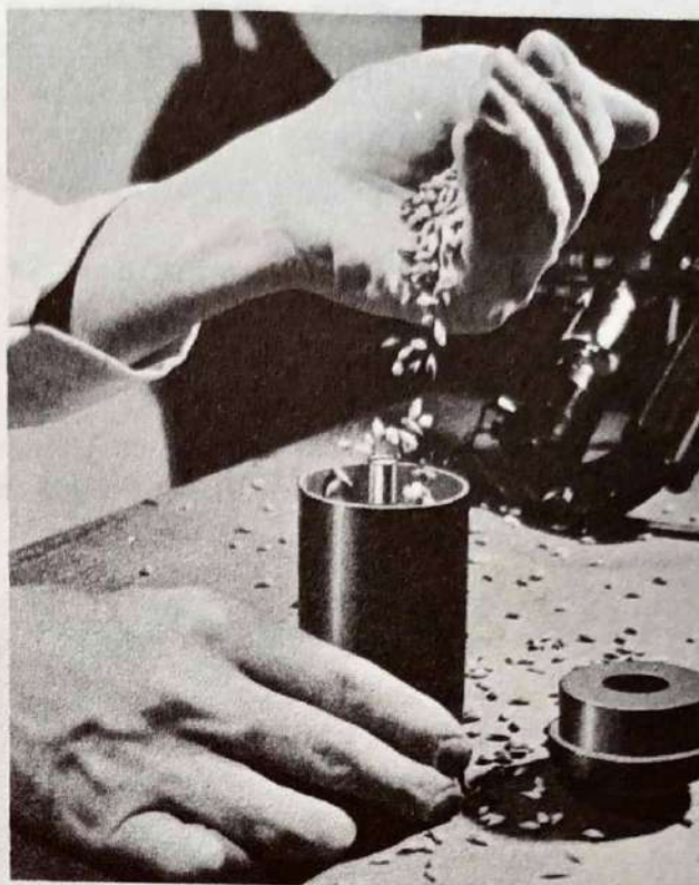
1 Remove the top and feed the sample into the upper cavity.
