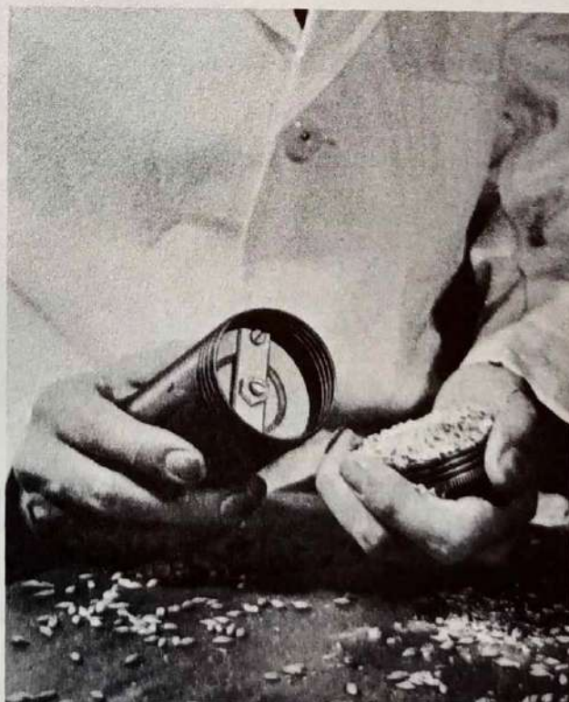
3 Unscrew the base to obtain the ground sample. (Screw inside lower cavity adjusts fineness.)
