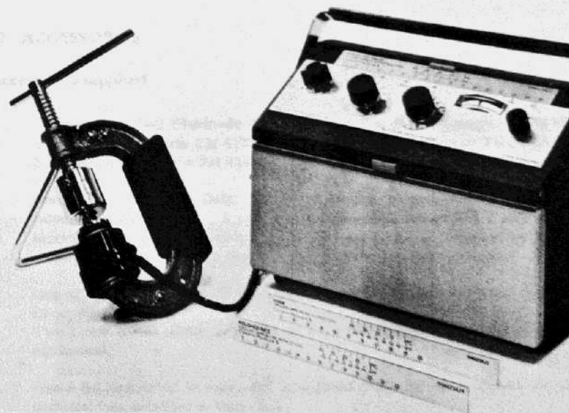
Fig. 1.1 The moisture meter with compression cell electrode and calculator scale fitted
