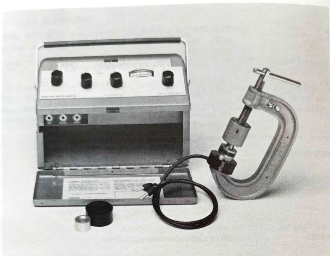
Fig. 1.2 The moisture meter showing accessories
